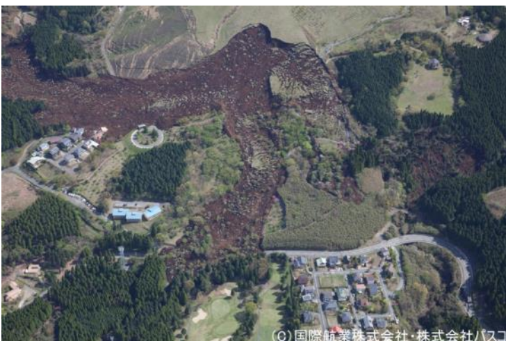
Fig. 9 Landslide flows on gentle slope of the lava dome. Landslide slip would have occurred in the tephra which covered on the lava.(View from point B in the Fig. 7)
